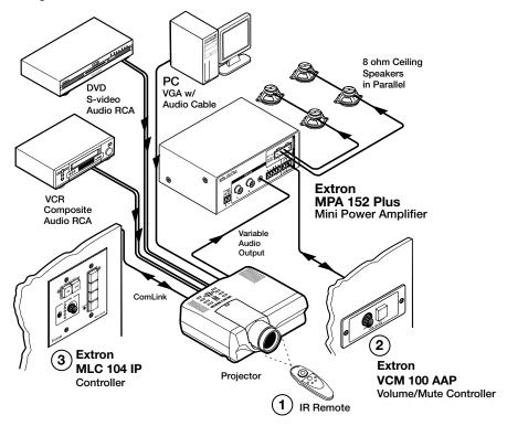
Figure 9. Typical Application for the MPA 152 Plus, Using Remote Control
